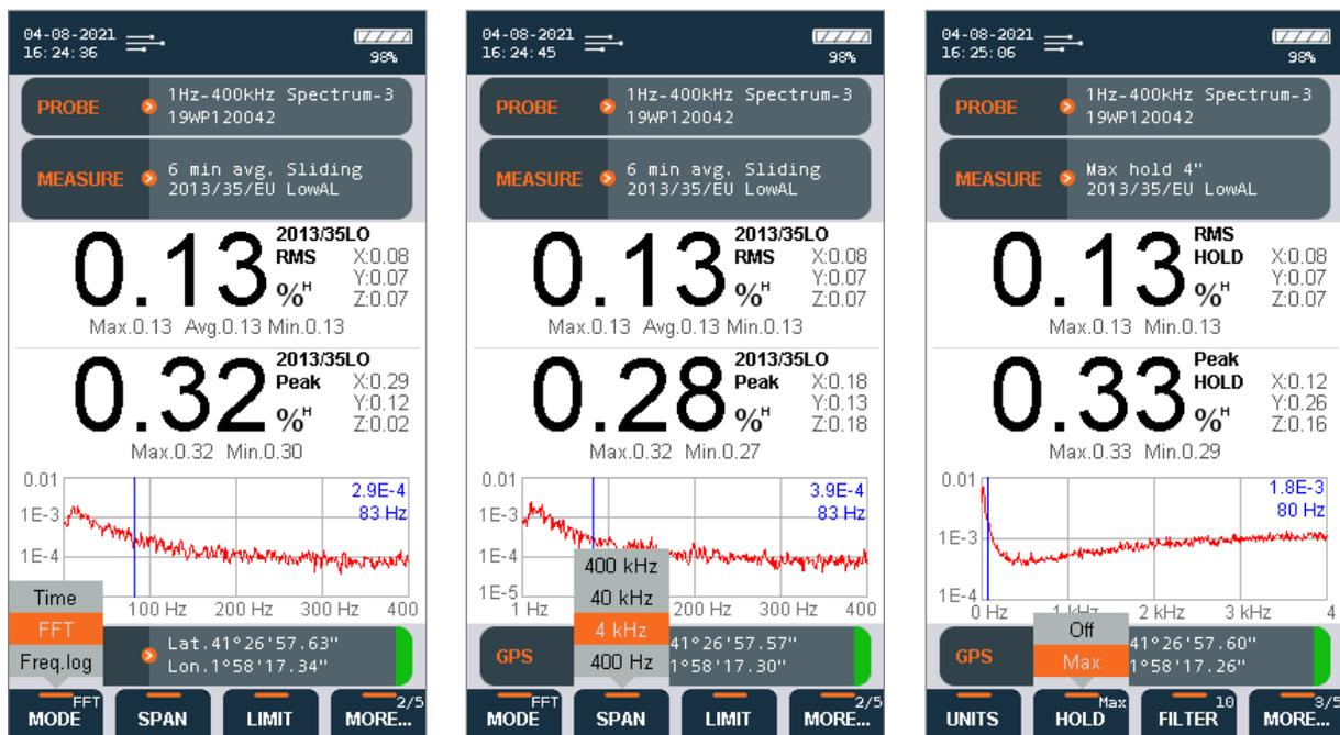
Figure 6. SMP series meter Menu Selection (a) FFT mode (b) SPAN (c) HOLD to Max
