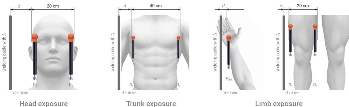
**Figure 2.** Areas for measuring EMF exposure in manual welding processes
