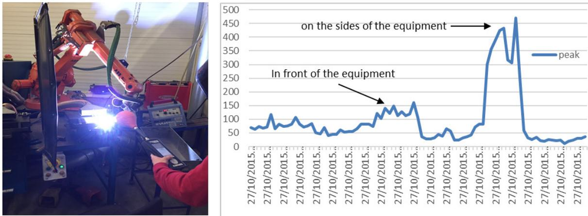
**Figure 10:** (a) Measurement of an ongoing welding operation (b) Comparison of measurement results in front of the equipment and on the sides of the equipment
