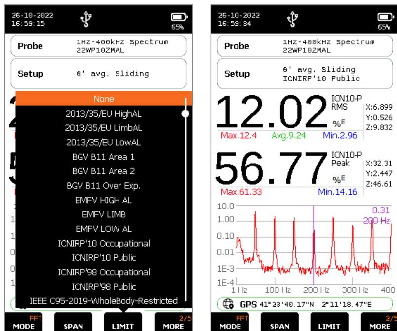
Figure 6. SMP3 screen with %ICNIRP value WPM
