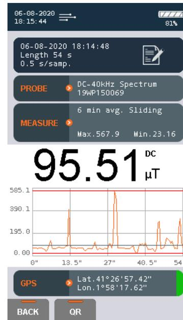
Figure 13: Final results for static field measurement.
