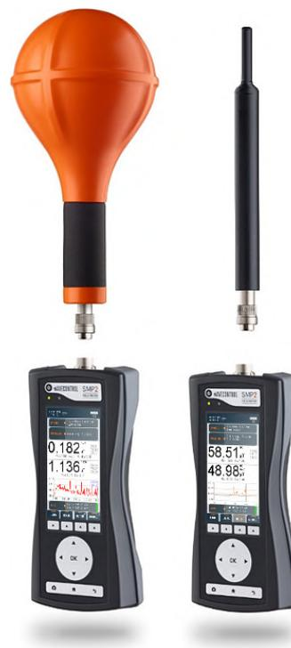
Figure 12: SMP2 EMF meter combined with the WP400 (1 Hz – 400 kHz) probe for AC magnetic field measurements (left) and the WPH-DC (DC – 40 kHz) probe for static magnetic field measurements (right).
