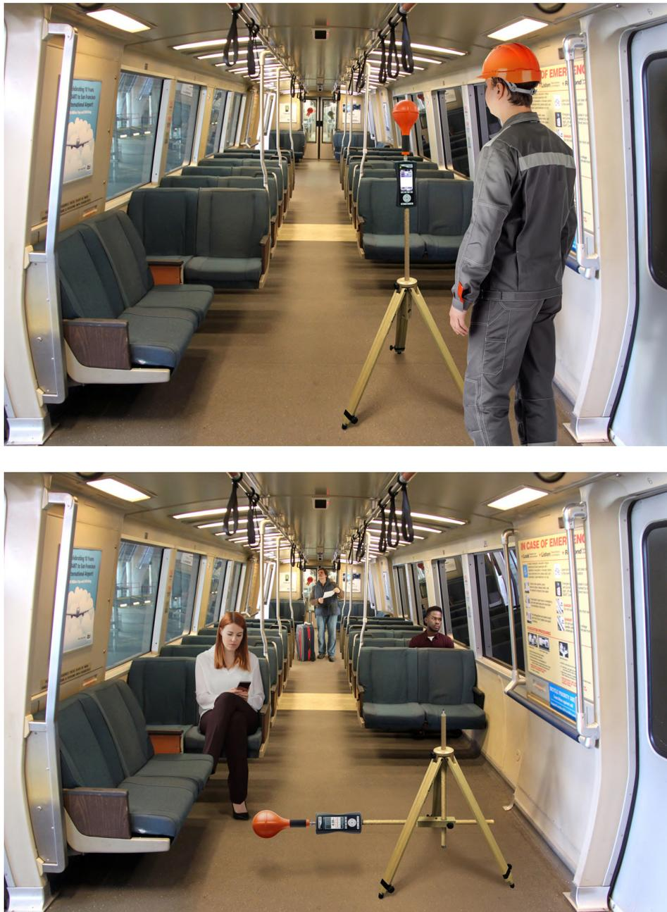
**Figure 3:** SMP2 mounted on a tripod at 1.5 m (top image) and at 30 cm distance from where the public may be for assessment in public areas. Using the horizontal extension, the SMP2 can also be placed on the tripod disk at a height of 0.3 m (bottom image).
